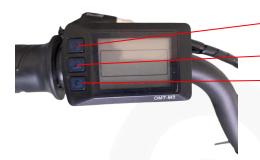
Increase power assist from 1 to 1.2/1.4/1.6/1.8 Press 5 seconds to turn on the front/rear light
