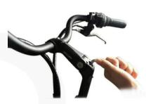
Adjust the tilt of the handlebar to a comfortable position ranging from 40° to -10°, then tighten with socket head wrench.
