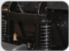
Shock absorber Adopting automobile steering system design,independent suspension system
