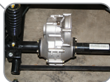
Transaxle Continuously variable transaxle no noise
