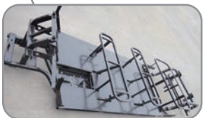
Chassis High tensile steel welding structure, electrophoresis treatment for the whole chassis enhances the anti-corrosive and anti-rust performance
