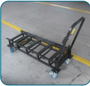
Push-pull type battery loading and unloading frame
