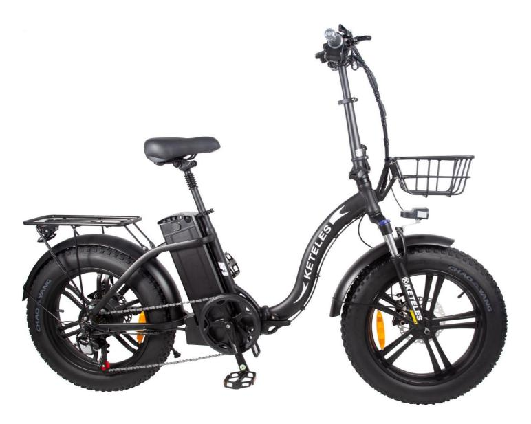
Model: KF9-B 20" Folding E-Bike 48V 1000W Rear Hub Motor 48V 23AH Lithium Battery 20"x4.0" Fat Tire
