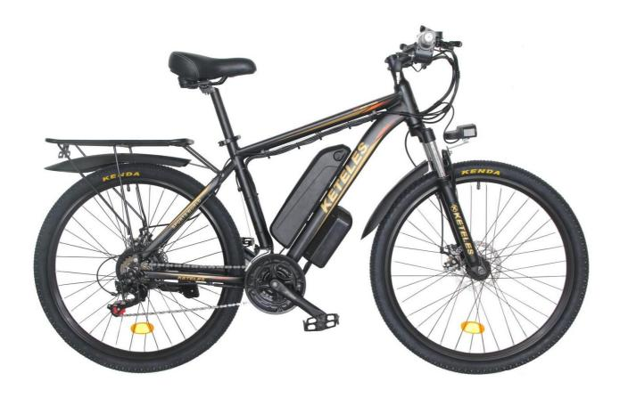
Model: K820 Mountain E-Bike 48V 1000W Rear Hub Motor 48V 17.5AH Lithium Battery 26"x1.95" MTB Tire ( can also be made 29" Dual Motor version )
